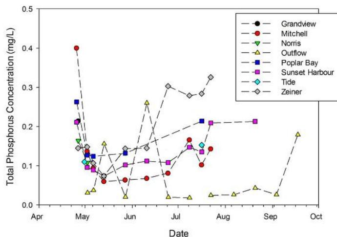
Figure 1: Total phosphorous concentration in inlet and outlet streams (ref. Teichreb 2013 p.30)
