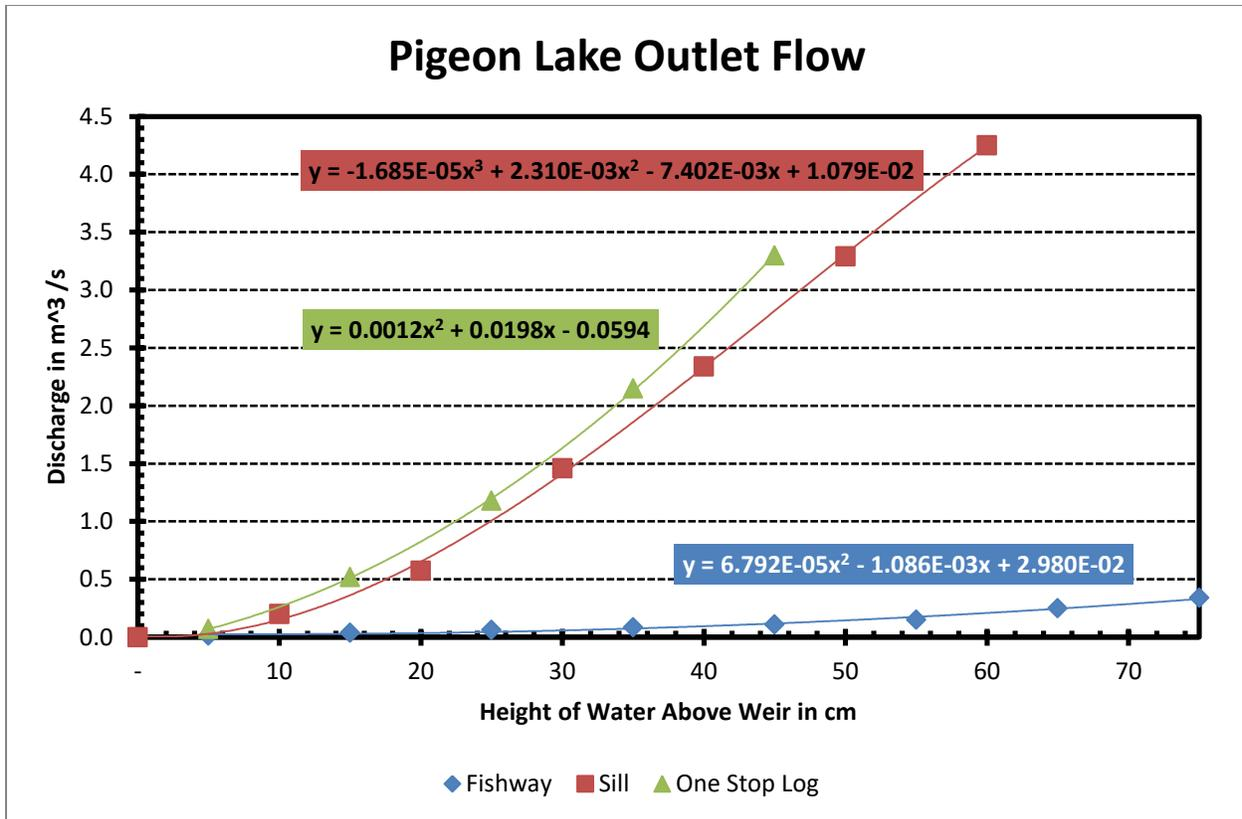
Figure 4. Pigeon Lake Weir discharge curve
