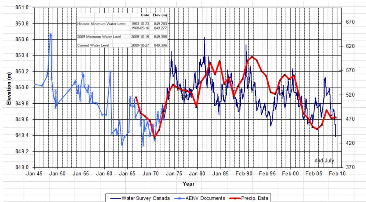
Figure 6. Comparison of variation in Pigeon Lake elevation to rolling average 5-year precipitation
