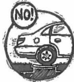
**Don't** drive over your tank or any buried components in your system, unless they've been equipped with a special traffic lid. If the system is subject to possible traffic, put up a barricade or a row of shrubs.
