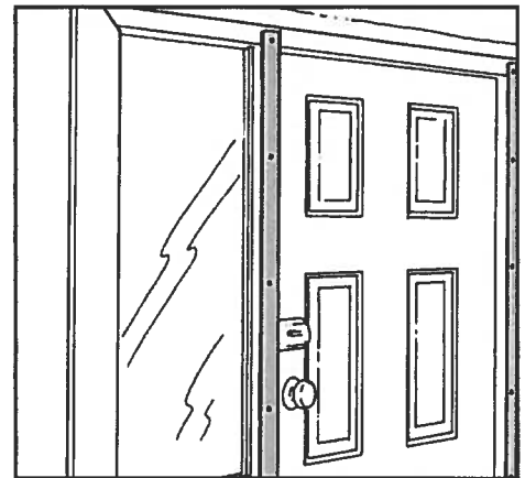
Figure 5 Use long screws to install metal brace on frame of door with sidelights.
